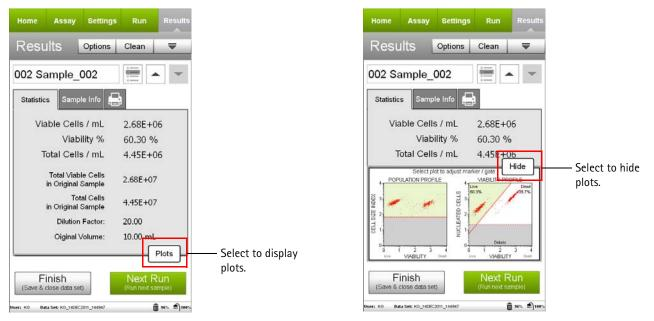
12. (Optional) If changes are needed to the cell size gate or viability marker, touch a plot to enlarge it, then adjust the cell size gate and/or viability marker as described in steps 4 and 6. You cannot adjust the nucleated cells threshold after the sample has been acquired.
