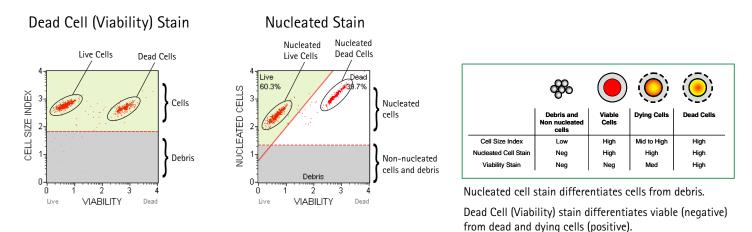
Each plot has moveable markers. The first plot has a gate marker, allowing you to eliminate debris based on size. The second plot also has a threshold marker, allowing you to eliminate cells that do not have a nucleus. This plot also has an angled marker (viability discriminator), allowing you to separate live cells from dead cells.
