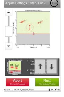
This example data show typical gate and marker settings. The threshold was raised to remove debris.
