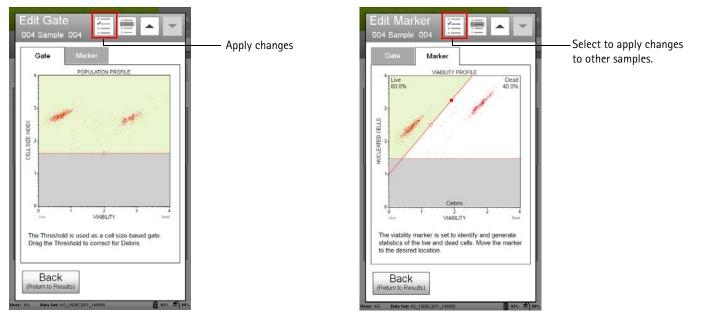
13. If no adjustments are needed, select Next Run and repeat steps 9 through 12 for the remaining samples.
